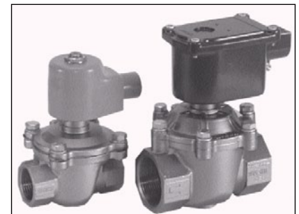
Fig. 3: Mains 230V AC 2/2-way semi-pilot, diaphragm type, solenoid valves
