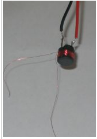
10mH choke with 150 turns for the secondary
